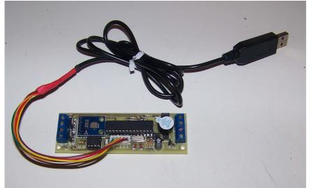
The altimeter should be beeping away doing its continuity test. A beeping altimeter does not mean an established communication.
